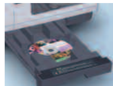
An additional drawer allows the removal of individual discs. This makes problems due to unreadable discs easy to resolve.
